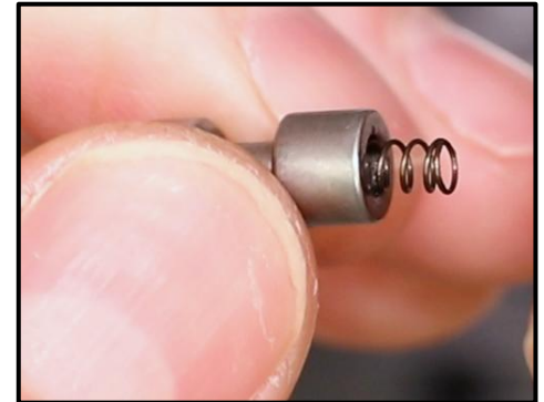
Step 16: Put some Synthetic Grease on the new Striker Block Safety. Insert it into the Striker Block Safety.
