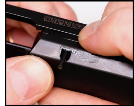
Step 28: Use your Hammer and Bench Block to Tap in the Extractor Pin the rest of the way.
