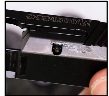
Step 28: Use your Hammer and Bench Block to Tap in the Extractor Pin the rest of the way.
