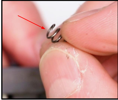
Step 26: Keeping the Striker Block Safety Compressed, Insert the Extractor. Make sure the Extractor Spring Locates in the small pocket on the Extractor.
