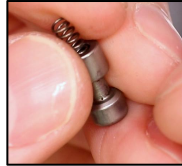
Step 16: Put some Synthetic Grease on the new Striker Block Safety. Insert it into the Striker Block Safety.
