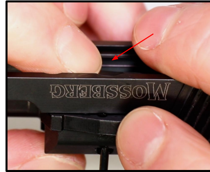
Step 28: Use your Hammer and Bench Block to Tap in the Extractor Pin the rest of the way.
