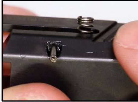
Step 26: Keeping the Striker Block Safety Compressed, Insert the Extractor. Make sure the Extractor Spring Locates in the small pocket on the Extractor.
