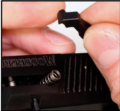
Step 26: Keeping the Striker Block Safety Compressed, Insert the Extractor. Make sure the Extractor Spring Locates in the small pocket on the Extractor.
