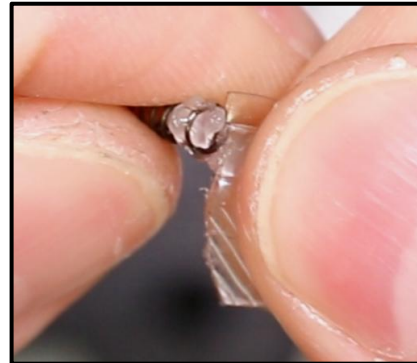
Step 16: Put some Synthetic Grease on the new Striker Block Safety. Insert it into the Striker Block Safety.
